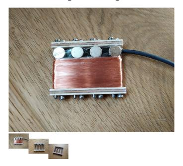
4-String Single Coil Pickup Dimensions BxHxT = 47x40x5.5mm
