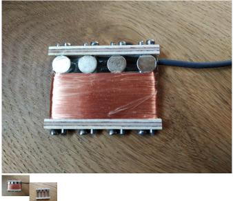
4-String Single Coil Pickup Dimensions BxHxT = 47x40x5.5mm
